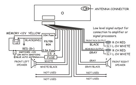
**CAUTION!** Tape unused wires so they do not short against other wires or chassis ground.
